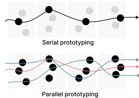
**Figure 2: Comparison of serial and parallel prototyping workflows: in serial prototyping, designers make sequential decisions, finalizing a single prototype (grey circles represent options, black circles indicate the choice). Parallel prototyping retains multiple options, enabling flexible combinations and simultaneous exploration of alternatives.**
